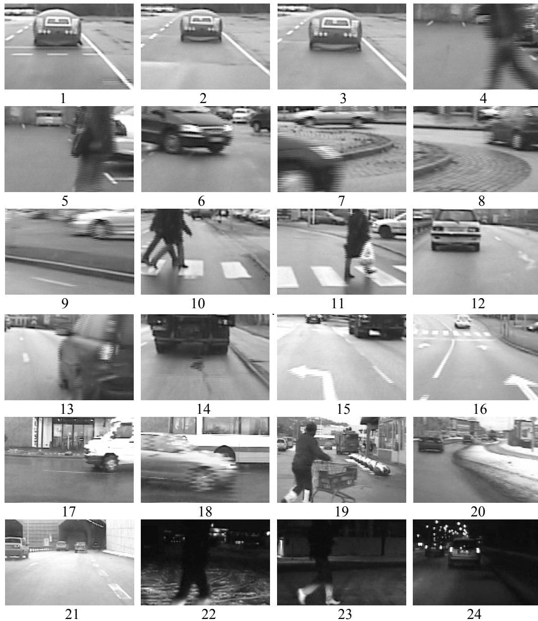
Figure 3. Samples of driving scenes for testing the collision detection system. 1-3 collision events, collision with car at three speed levels: relatively slow, mediate and fast respectively; 4-5 translating events, fast translating figures, while driving at low speed; 6-7 translating events, fast translating cars; 8-9 translating events, turning and translating cars, normal driving speed; 10-11 translating events, translating human figures; 12-13 translating events, car cutting in; 14 approaching but not collision event, driving after a truck; 15-16 translating events, road symbols, driving at high speed; 17-18 translating events, fast translating car/van; 19 translating man with a trolley; 20 translating event, turning; 21 driving into, in and out of tunnel; 22-23 translating events at night, pedestrians; 24 approaching but not collision event at night.
