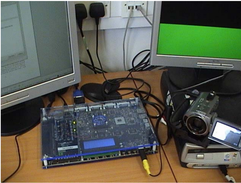
Fig. 9. The system setup includes a Celoxica RC340 board, a digital camera and two monitors. The modified LGMD model lights up the LEDs (flash lights) on the FPGA board based on the values of both LGMD and D cells. These values are also shown on the LCD of the FPGA board.
